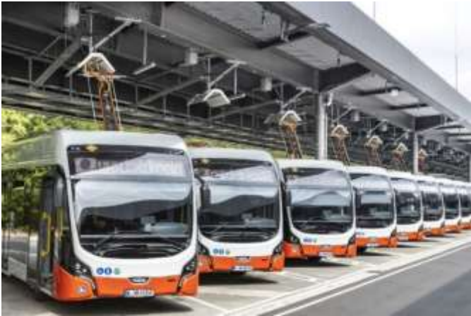
Figure 47 - Cologne’s operator KVB depot charging infrastructure for 51 BEBs since July 2021
